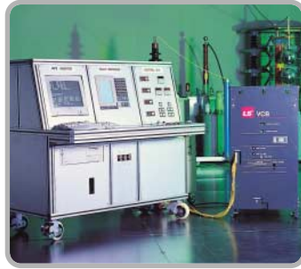
Characteristics Test / VCB Characteristics Test
